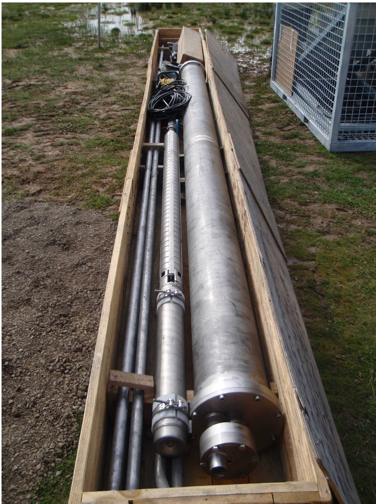
Photo 1: Crated ISD system (main treatment vessel, pump, steel rods and spare RO membrane element delivered to the Joel South site.
